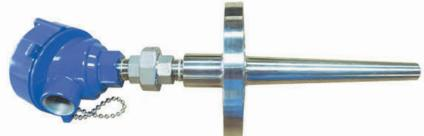
In most process applications the temperature sensor is inserted into a thermowell or protection tube. This protects the sensor from its environment and facilitates easy removal and replacement. These assemblies generally consist of a head, nipple-union-nipple and thermowell. Smart industrial thermocouples and RTDs are available in virtually any calibration and resistance temperature coefficient.
